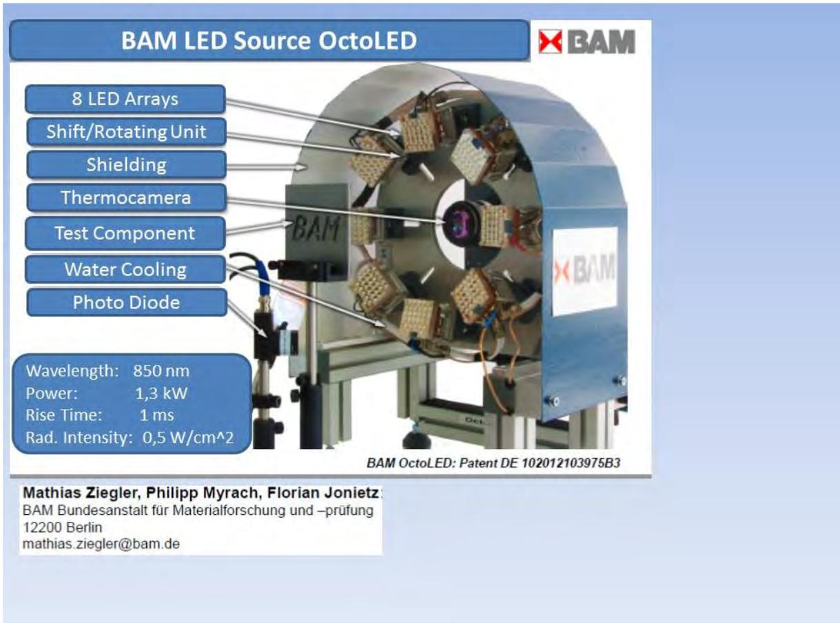
Fig. 4: Thermographic Testing by LED thermal excitation of the Test Specimen (BAM)
