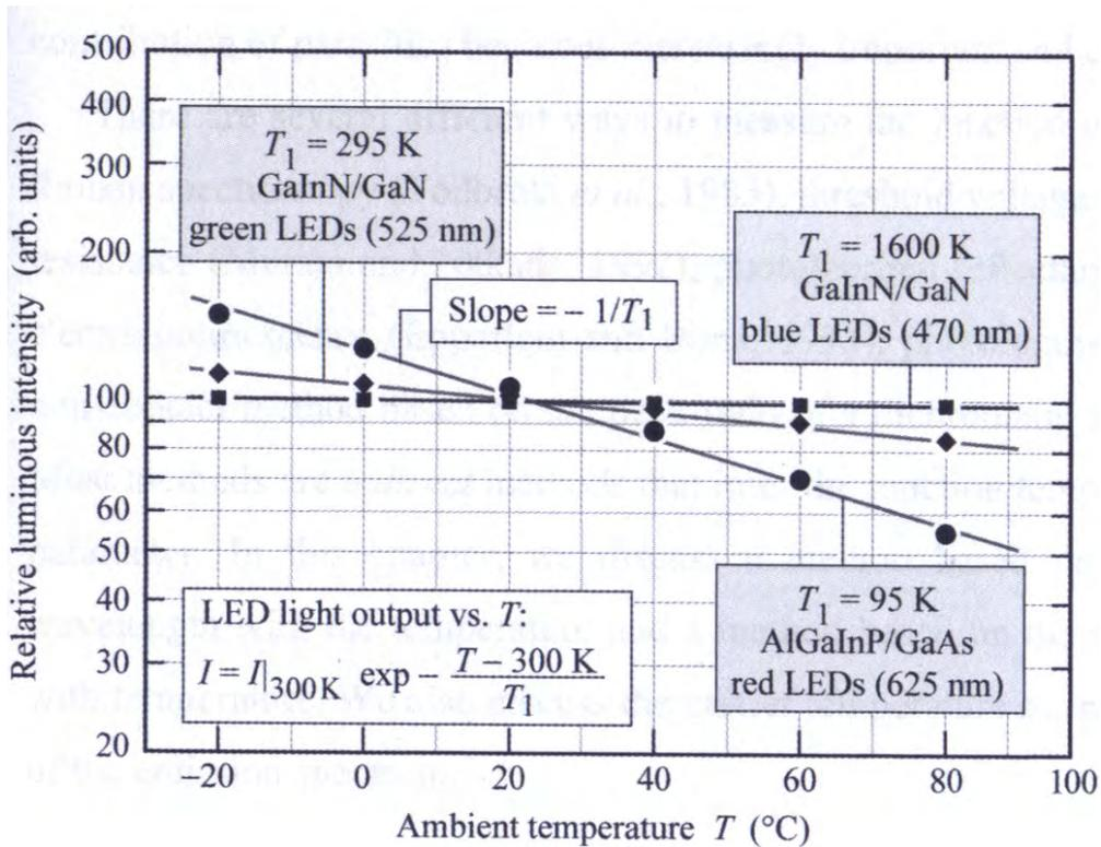
Figure 6: Temperature dependence of the luminous intensity of some LED semiconductor compounds [1,6]
