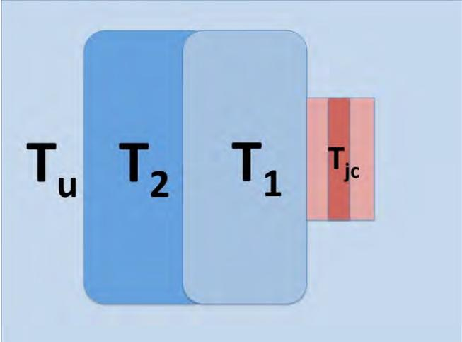
Fig. 8: Temperature management of LED; temperatures measured are: ambient  $T_u=28^\circ\text{C}$ , housing  $T_2=39.6^\circ\text{C}$ , LED heat sink  $T_1=42.7^\circ\text{C}$  and junction  $T_{jc}$ .
