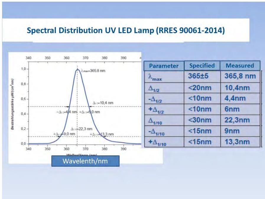
Fig. 9: Spectral Distribution UV LED Lamp, specification according to RRES 90061-2014, measurements at Helling Company
