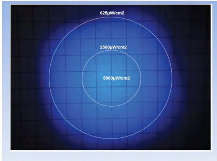
Fig. 11: Test with white paper (ASTM E3022 – 2015, RRES 90061-2014)
