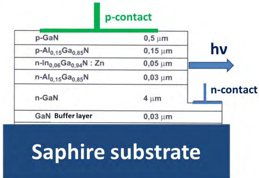
Figure 1: Schematic drawing of the first blue LED by NICHIA corp
