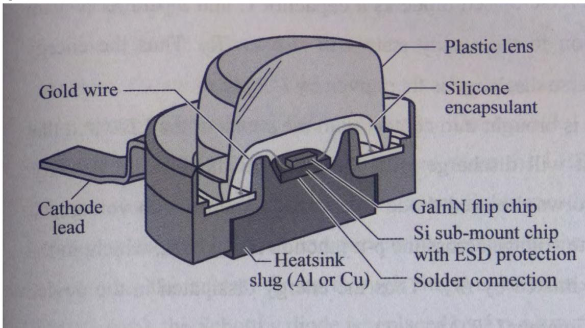
Fig. 7: Schematic drawing of the design of a high power LED [1]
