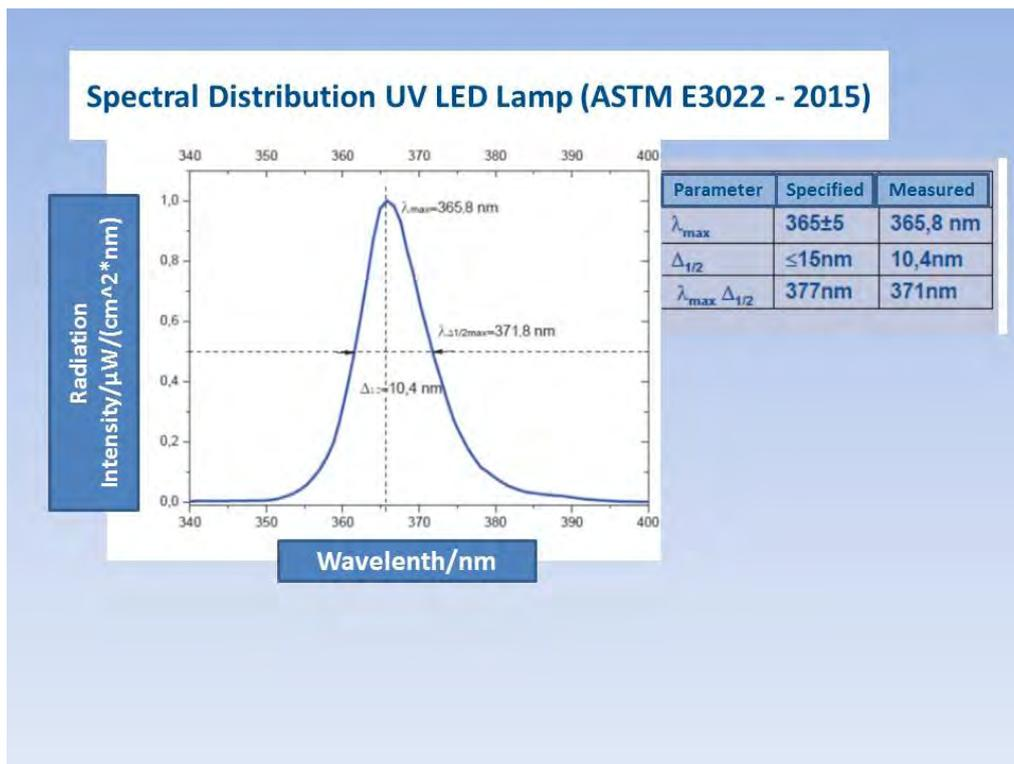
Fig. 10: Spectral Distribution UV LED Lamp, specification according to ASTM E3022: 2015, measurements at Helling Company
