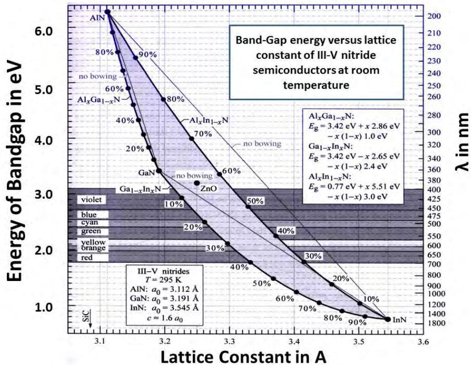
Figure 3: Bandgap energy and wavelength of emitted photons versus lattice constant in Angstrom (Å) of III-V nitride semiconductors at room temperature [4,5].
