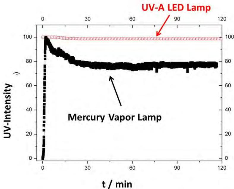
Figure 12: Warm up time for Mercury Vapor and LED UV-A lamps
