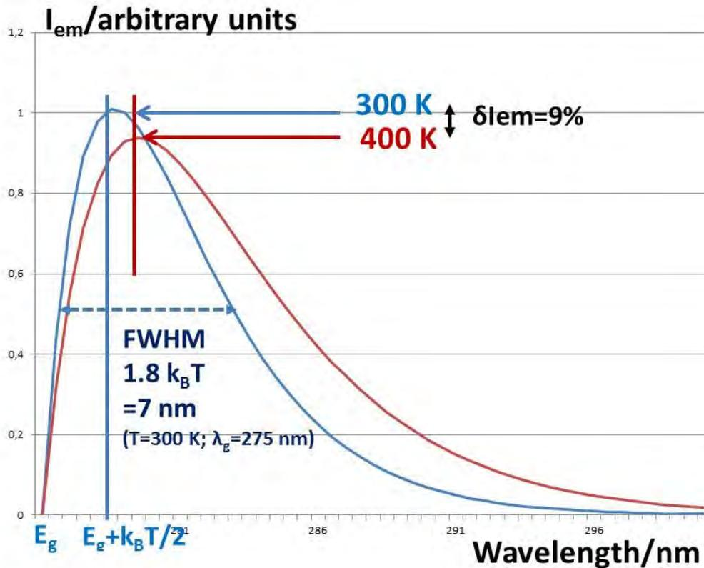
Figure 5: Emission spectra of direct emissions in LED,  $\lambda=275$  nm
